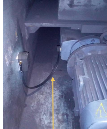
AsystemSentinel beacons in situ - their smart probe allowing set up in tight spaces
